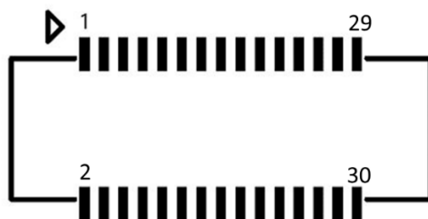
Figure 2.2. XM126 J2 connector footprint.
